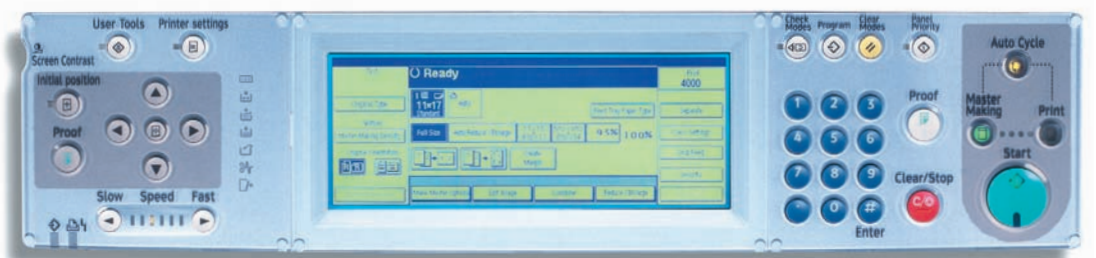
The new, large LCD panel makes it easy to print any job and program frequent functions.
